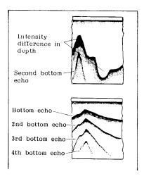
The width of the bottom echo can be used to help determine the density of the bottom material (soft or hard). The harder the bottom, the wider the trace. If the gain is set to show only a single bottom echo on mud, a rock bottom will show a second or third bottom return. The Basic Range chosen should be set to show the first and second bottom echoes when bottom hardness is being determined.
